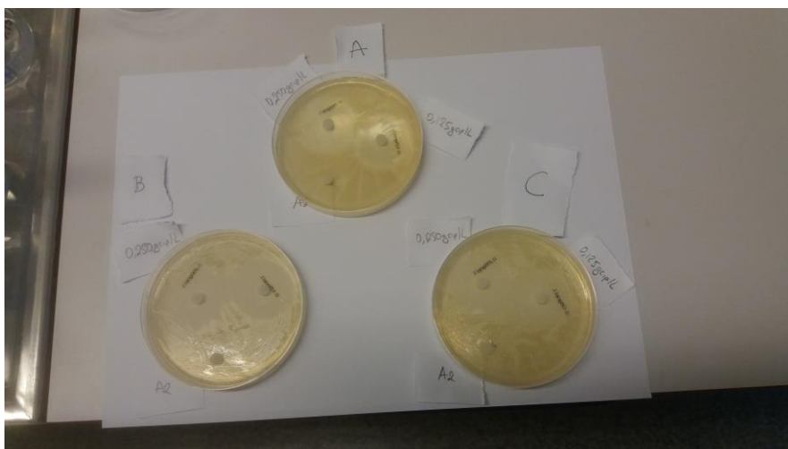
Picture 17: Plate A,B and C that contains 3 disks with 0,250g cip/L, 0,125g cip/L and sample A2.
